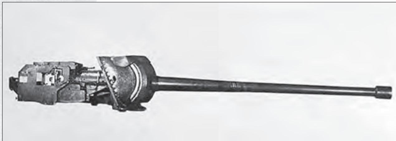
S-26-1 122 mm SP gun developed by TsAKB as part of the program to counter Germany's menagerie of weapons (TsAMO).
