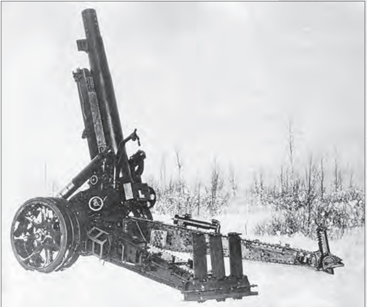
M-40 203 mm howitzer during testing, gun in firing position (TsAMO).
