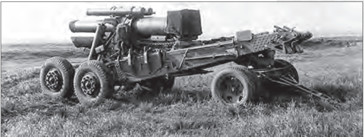
U-3 203 mm corps-level heavy howitzer in travel position (TsAMO).
