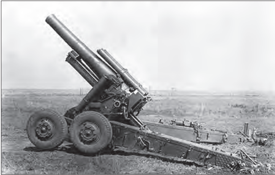
U-3 203 mm corps-level heavy howitzer elevated to 45 degrees. This gun was developed to replace the B-4 howitzer and was proposed several times for installation in an SP gun (TsAMO).
