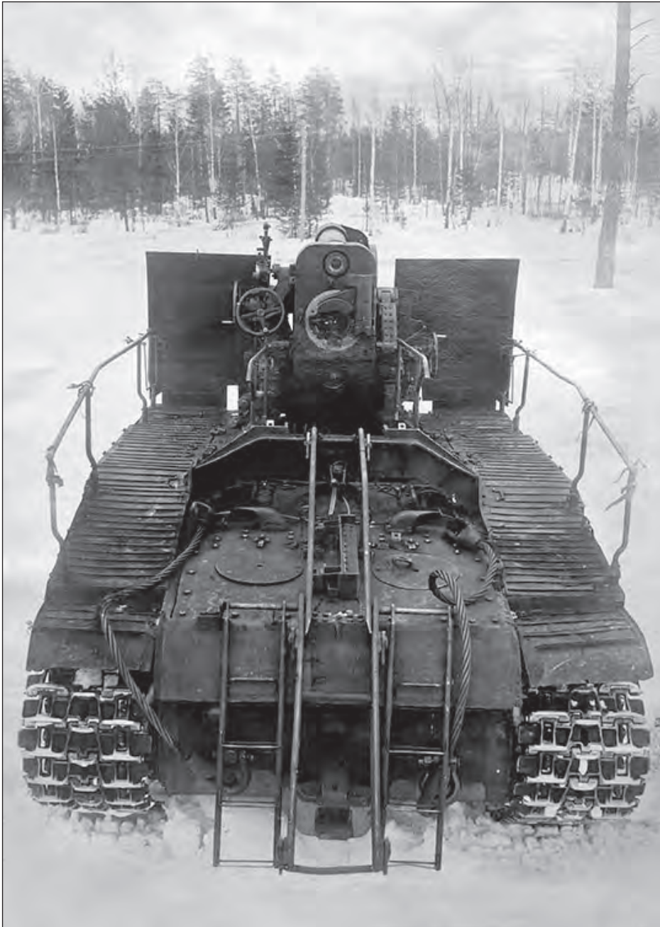
Rear view of S-51 SP gun. The fold-out ladders and guide rails for the loading tray are clearly visible (TsAMO).
