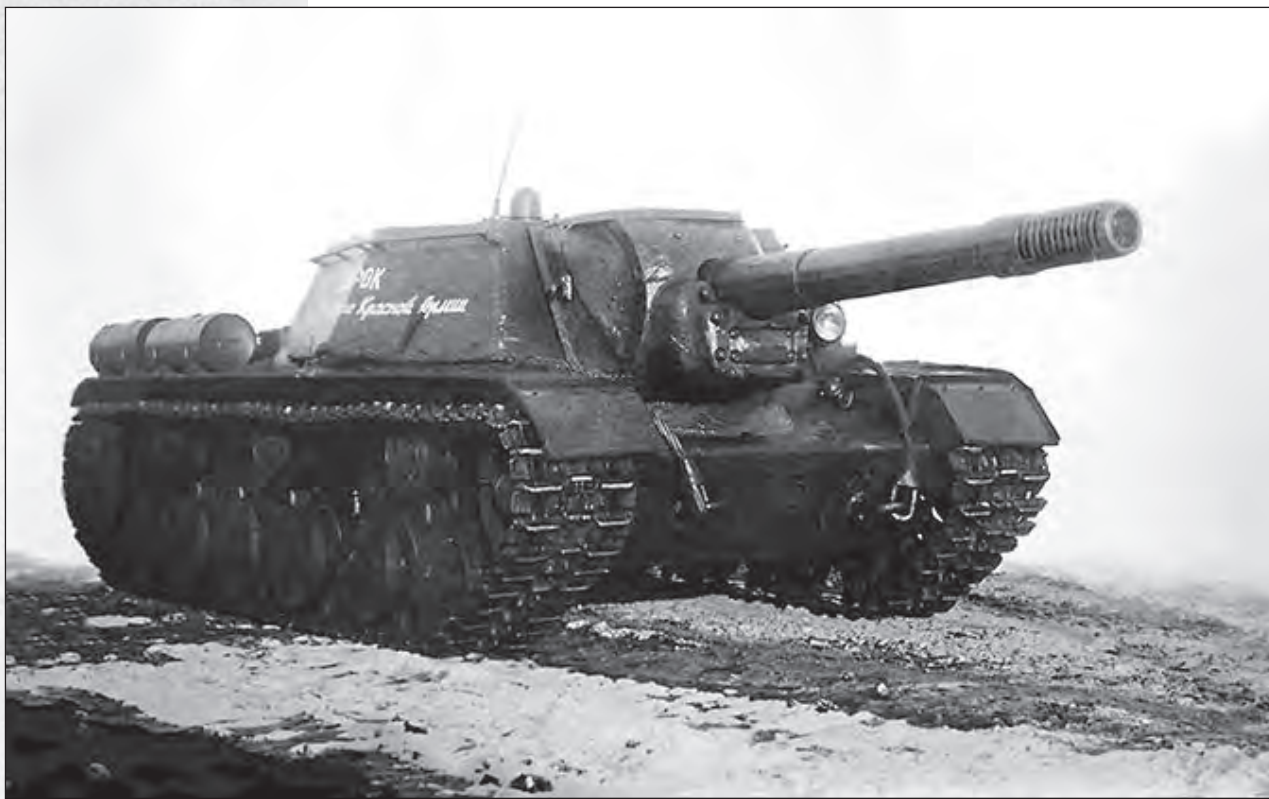
KV-14 SP gun prototype, late January 1943 (TsAMO).
