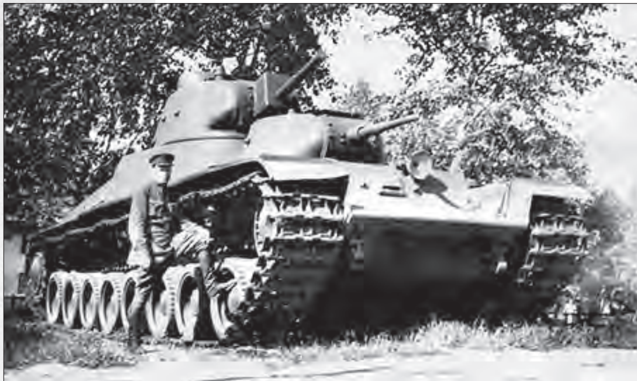
The T-100 heavy tank served as the base chassis for development of the first specialized bunker buster (V. Len).
