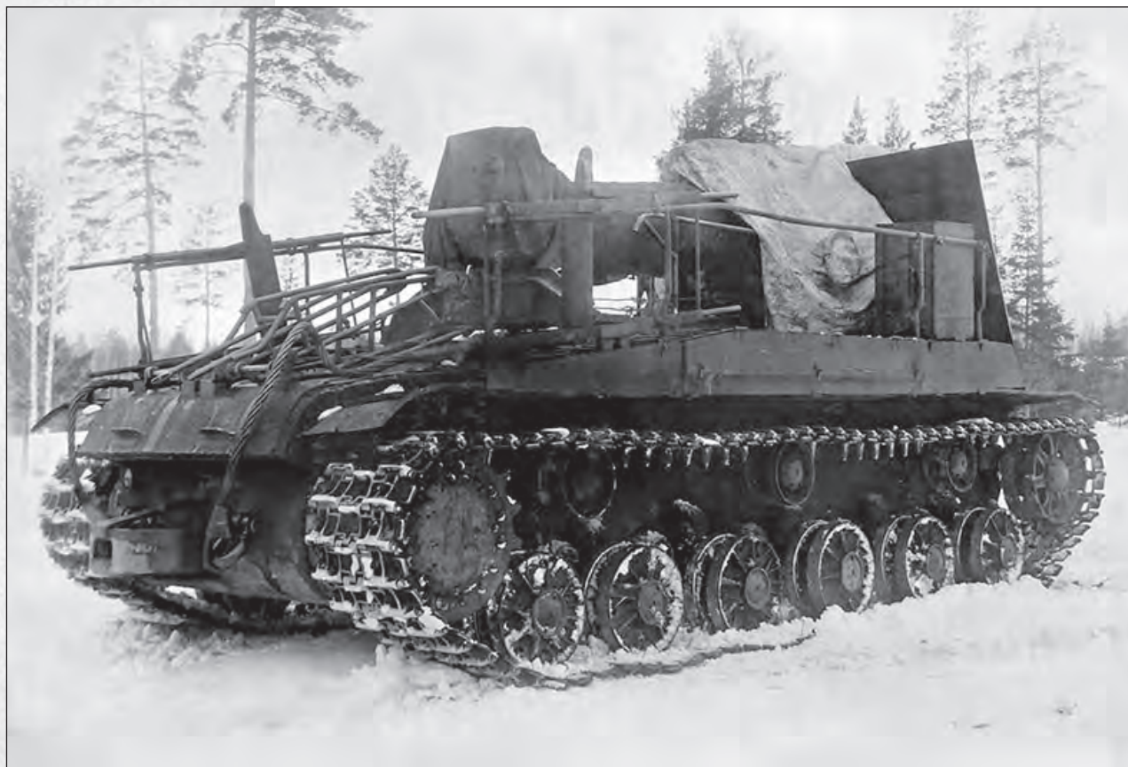
Rear view of S-51 203 mm SP gun in travel position (TsAMO).
