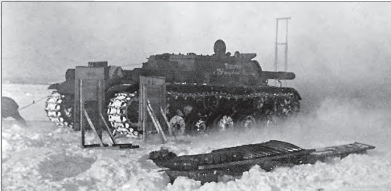
KV-14 undergoing test firing. For safety reasons, the first few rounds were fired without the crew in the superstructure (TsAMO).
