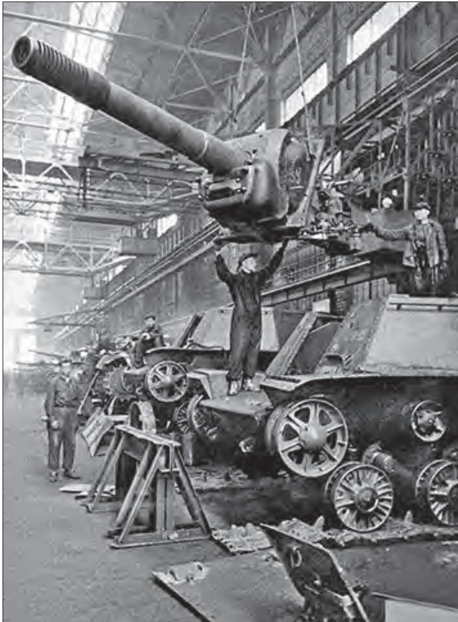
Mounting an ML-20S on an SU-152 SP gun (RGAKFD).
