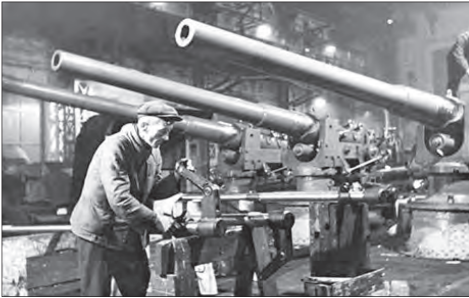
B-13 130 mm naval guns undergoing assembly at the Bolshevik Factory. This gun and others with its ballistics were frequently used as armament for SP guns (V. Len).
