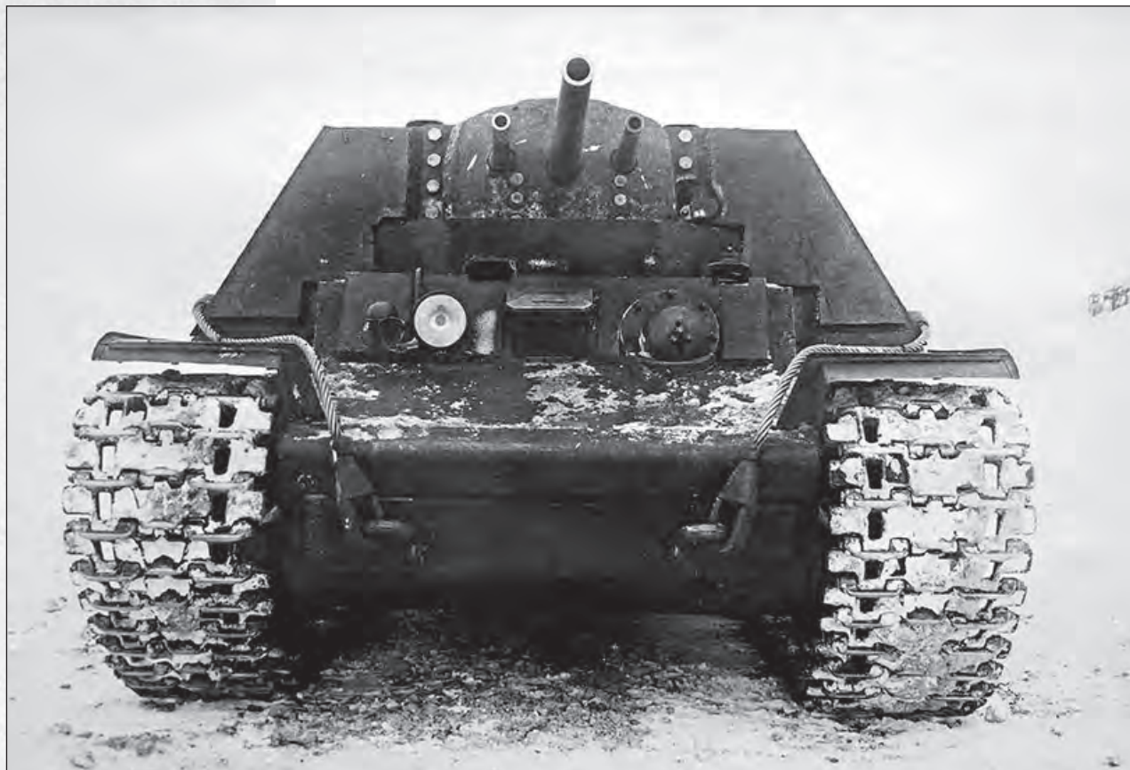
Front view of a KV-7; the tank's massive mantlet and the skirt underneath it are clearly visible (TsAMO).
