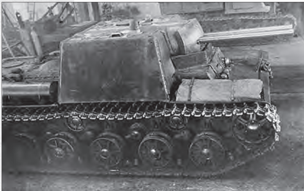
KV-7 assault tank with U-14 twin gun system, Chelyabinsk, spring 1942 (IZh).
