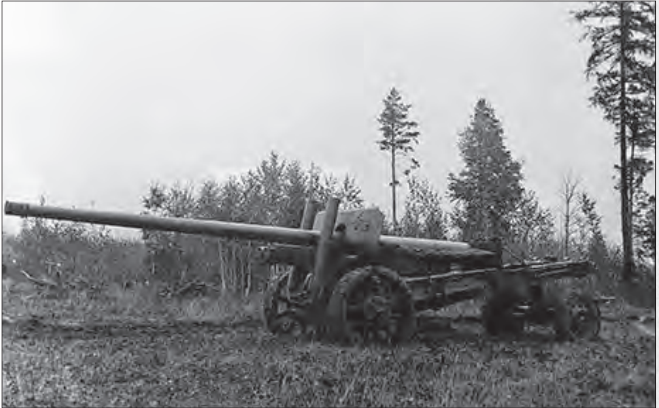
M75 107 mm antitank gun in travel position (TsAMO).
